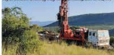
Exploration for Uranium by Truck Mounted Hydrostatic Drilling Rig in Tummalapalle area, A.P.
