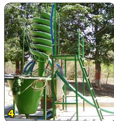
Xenotime bearing concentrate Recovery Plant, Chhattishgarh
