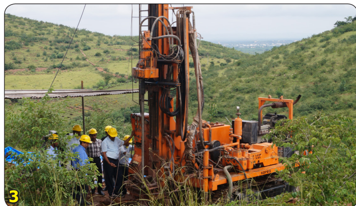
Sub-surface exploration by crawler mounted Hydrostatic Rig (Departmental)
